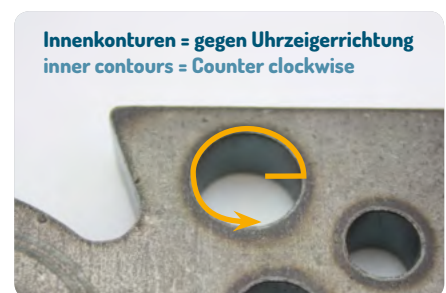
Schneidablauf Innenkonturen Cutting process for inner contours
