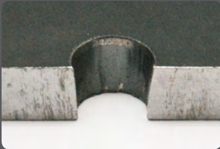
Plasmaschneiden ohne Contour Cut Plasma cutting without Contour Cut
